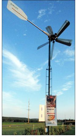
pended above the bottom of the 90-foot well. The compressed air, being lighter than water and under pressure from the overlying water column, expands as it "lifts" the water up the plastic piping and fills the 500-gallon tank 15 feet above the ground.
